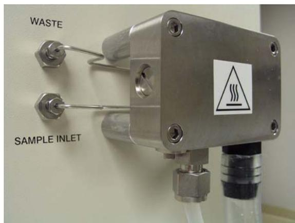
Figure 20: The Sample Inlet Block
